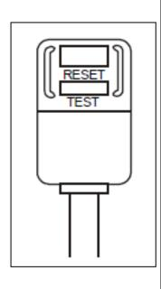
Your portable air conditioner is supplied with a Leakage-Current Detection and Interruption (LCDI) plug. This plug reduces the risk of fire due to arcing faults in the power supply cord. Please follow the instructions below to ensure that LCDI plug works properly.
