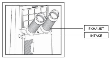
If installing the optional air intake hose in an area with poor air quality, we recommend purchasing the intake hose pre-filter accessory.
