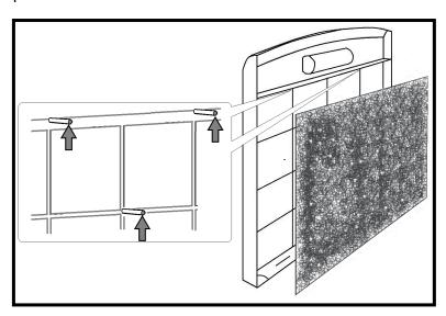
3. Once the activated carbon filter is secured, insert the assembled filter frame into the unit.
