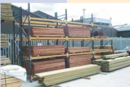
A fencing rack which is made from joining 2 frames together to make the rack twice as deep as a standard one
