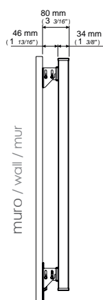
Ingombro con attacco corto Measurements with short wall brackets Mesurations avec attache court
