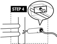
STEP 4: Guide the electrical cord through the electrical connection mounting tube (b) and use the long mounting screw (e) to tighten the electrical connection mounting tube to the vertical bar.
