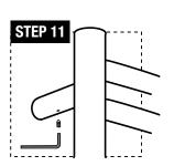
**STEP 11:** As shown in the picture, install the set screws (c) into the hole of all the tubes (a and b) using the allen wrench; fix the tube (a) onto the mounting bracket (g).
