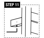
**STEP 11:** As shown in the picture, install the set screws (c) into the hole of all the tubes (a and b) using the allen wrench; fix the tube (a) onto the mounting bracket (g and h).
