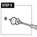
**STEP 9:** Insert long screw (i) through mounting bracket (g), then screw into plastic drywall anchor (f).
