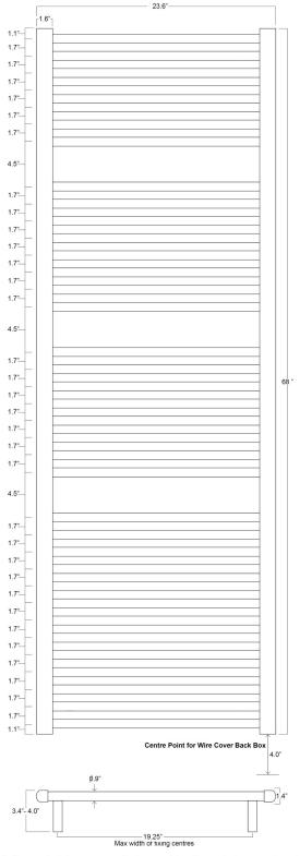
Position mounting brakets as near to each edge as possible and between the first or second cross bars
