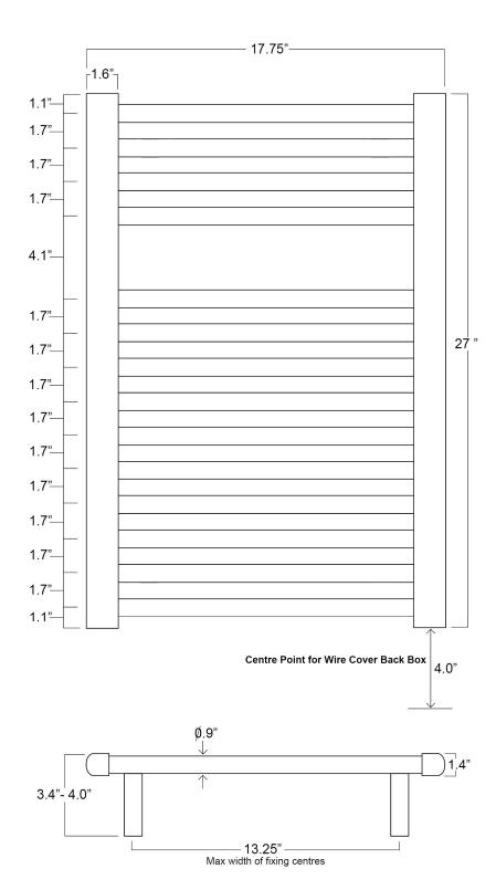
Position mounting brackets as near to each edge as possible and between the first or second cross bars
