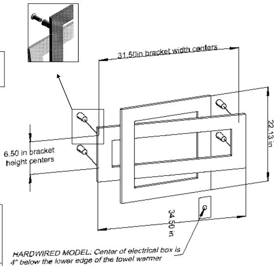
NOTE: Towel warmer *must* be installed so that electrical cord comes out of the *BOTTOM RIGHT* of the unit.
