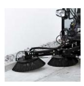
Side brush Makes work close to edges possible while increasing the area coverage of Kärcher sweepers.
