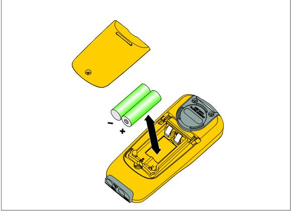
Figure 4. Battery Replacement
