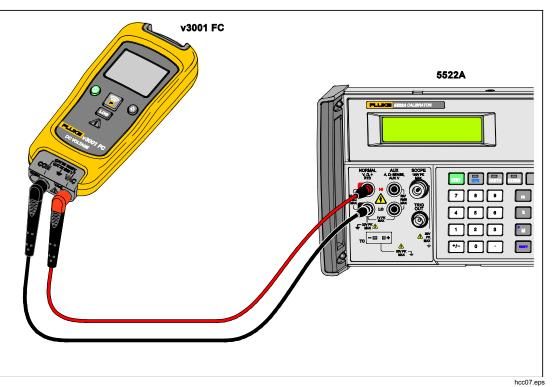
Figure 2. Performance Test Connections
