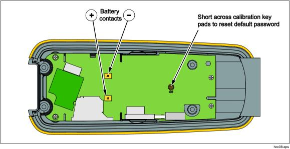
Figure 3. Calibration Password Reset
