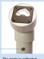
The meter is calibrated 0-100 to indicate a peak response to the Pulse Transmitter signal
