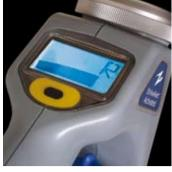
In the R mode the SuperC.A.T detects VLF radio signals re-radiated by buried metallic pipes and cables.
