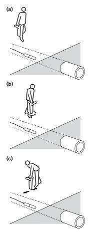
Propel the sonde a further three to four paces along the drain or duct and pinpoint and mark. Repeat this procedure along the route at similar intervals. It should only be necessary to change the locator sensitivity while tracing the sonde if there is a change in the depth of the drain or duct, or the distance between locator and sonde.
