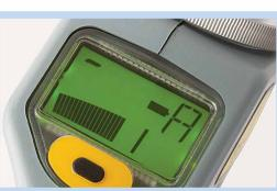
High contrast display with auto-backlight Bargraph 'tidemark' enables operators to quickly spot and zero-in on a buried conductor.
