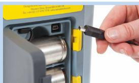
High speed USB 2.0 data connection Connect to a PC to configure C.A.T settings, run an eCert, and to rapidly transfer usage data from eC.A.T4 and gC.A.T4 series locators.
