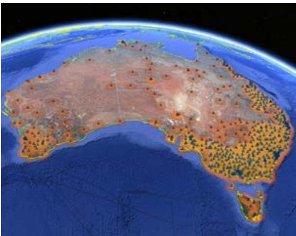
Each orange circle represents a RTK reference station. As of December 2013, the network comprised of more than 500 base stations.
