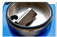
The air jet is rotating in a short distance close to the mesh of the test sieve. This results into a perfect Deagglomeration and dispersion of the particles.
