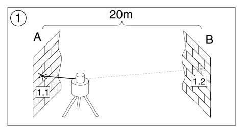
Now, place the unit near wall B with the plus X-axis pointing towards wall B. After the unit is level, mark the height of the laser beam at wall B. Turn the entire unit 180°, let it self-level and mark the center of the laser beam at wall A. The difference (h) of the marked points at wall A shows the deviation.
