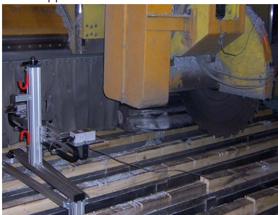
Fig 1: Gantry saw with Dimetix Laser
