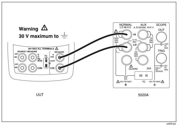
Figure 25. Isolated Voltage Input Calibration Connections
