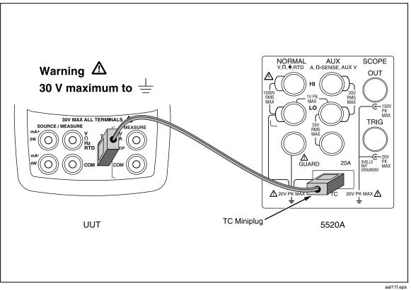
Figure 19. Thermocouples Calibration Connections
