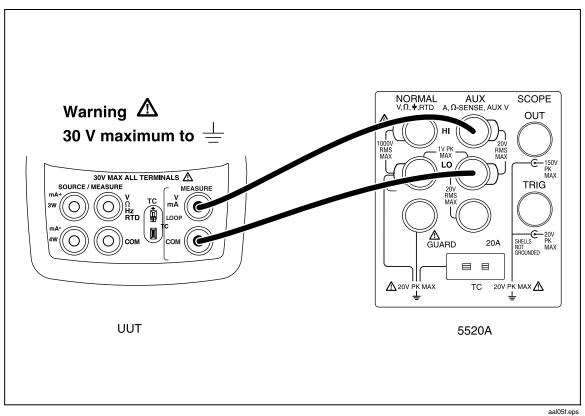
Figure 24. Isolated mA Input Calibration Connections
