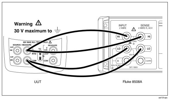
Figure 31. High Ohms Source Calibration Connections
