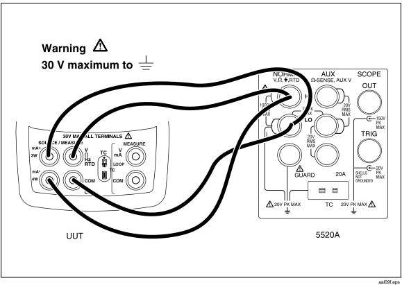
Figure 21. RTD Low Range Calibration Connections
