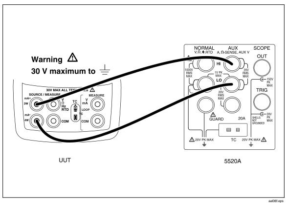
Figure 26. mA Input Calibration Connections
