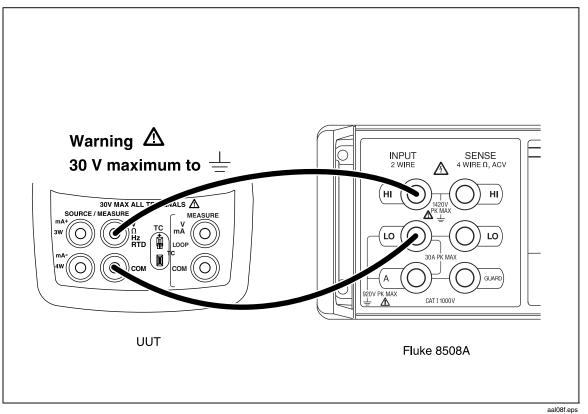
Figure 29. Voltage Output Calibration Connections
