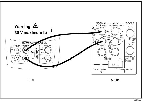
Figure 17. mV Input Calibration Connections
