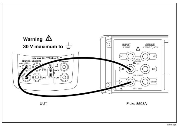
Figure 27. mA Output Calibration Connections
