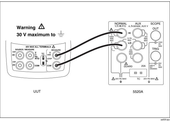
Figure 2. Upper Display Voltage Test Connections
