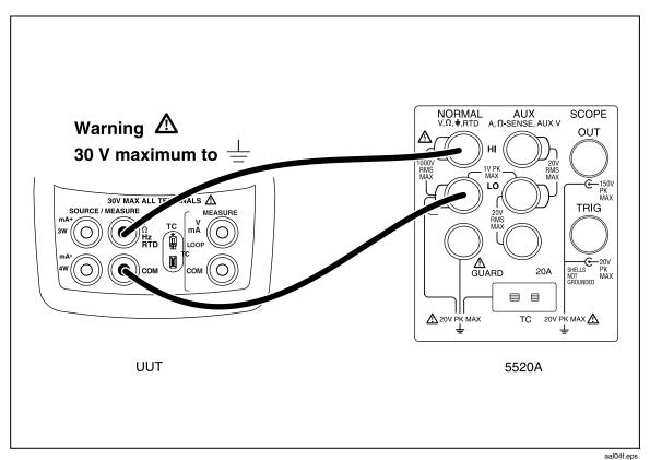
Figure 6. Lower Display Frequency Test Connections
