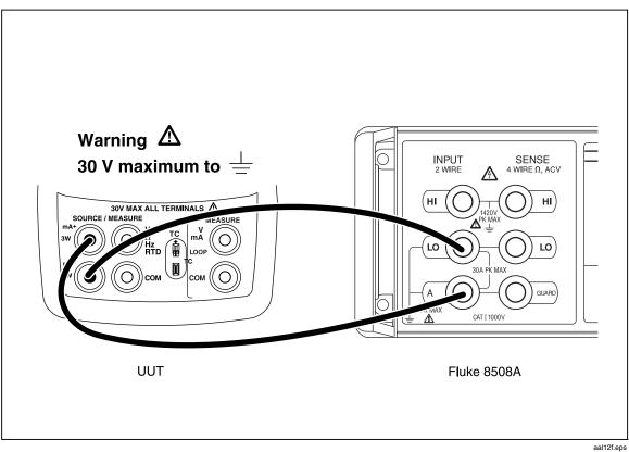
Figure 16. mA Output Calibration Connections
