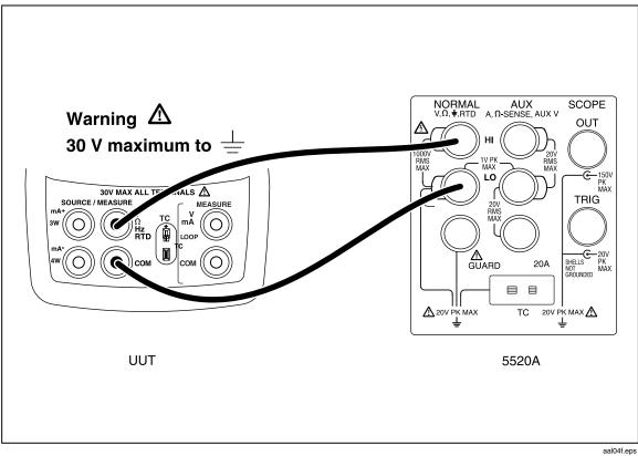
Figure 3. Lower Display mV and Voltage Test Connections
