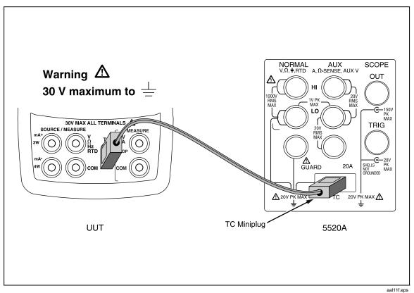
Figure 35. Thermocouple CJC Calibration Connections
