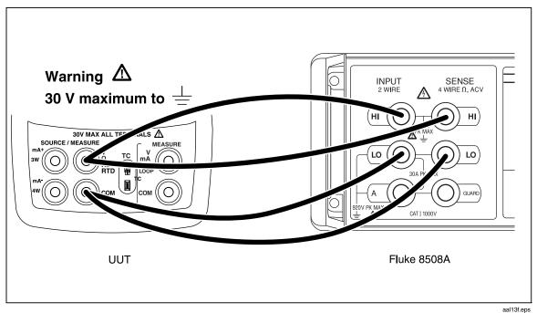
Figure 30. Low Ohms Source Calibration Connections
