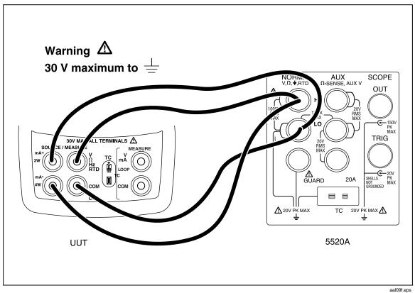
Figure 32. Ohms Measure Calibration Connections
