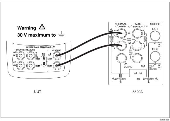
Figure 22. ISO Volts Calibration Connections
