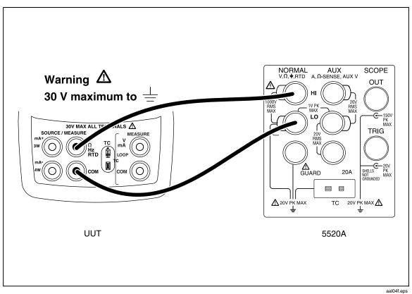
Figure 34. Thermocouple mV Input Calibration Connections
