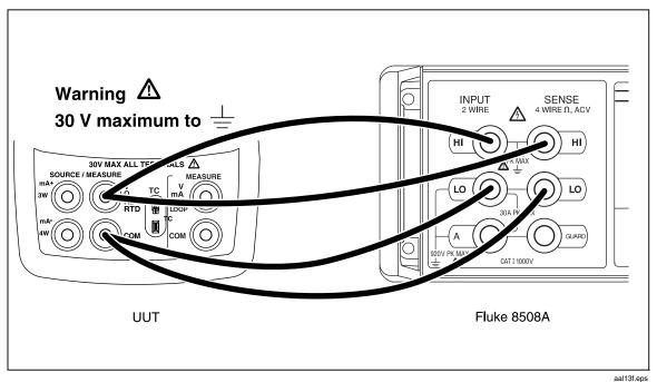
Figure 12. Lower Display Ohms Source Test Connections
