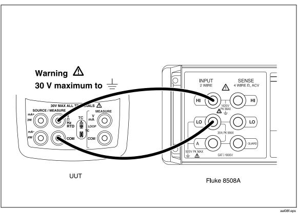
Figure 14. Volts Output Calibration Connections
