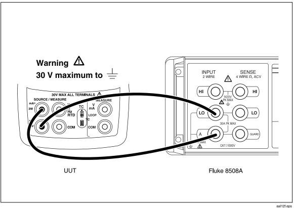
Figure 11. Lower Display mA Source Connections
