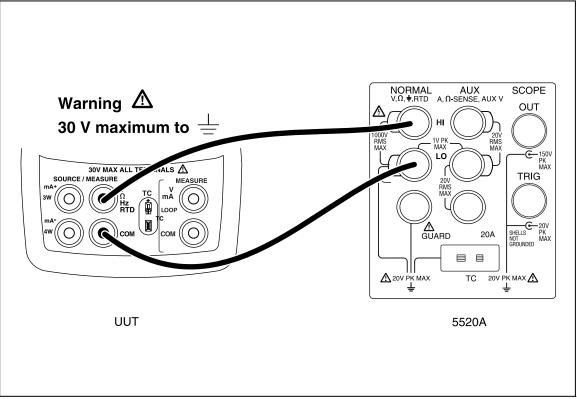
Figure 13. Volts Input Calibration Connections
