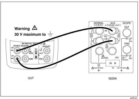
Figure 15. mA Input Calibration Connections
