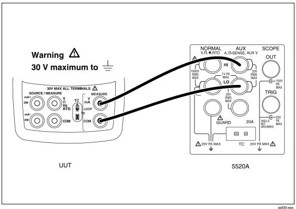
Figure 4. Upper Display mA Test Connections
