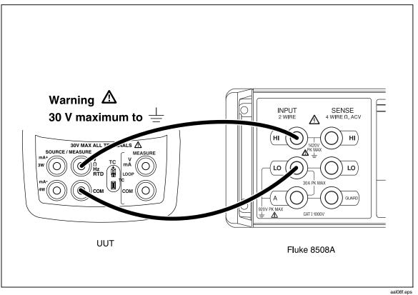
Figure 33. Thermocouple mV Output Calibration Connections
