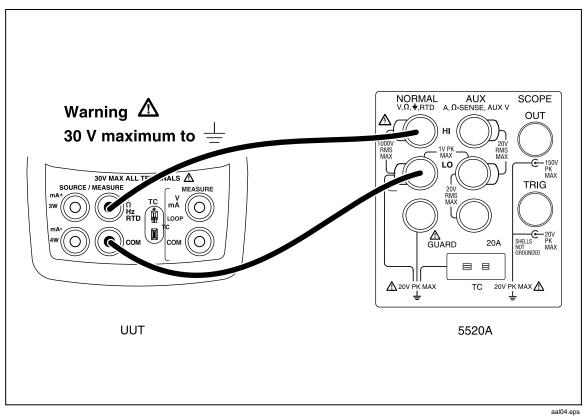
Figure 28. Voltage Input Calibration Connections
