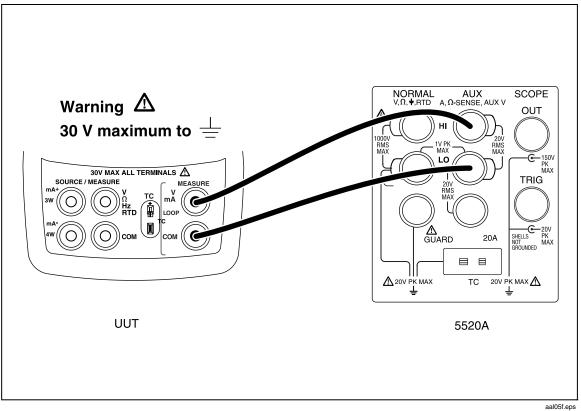
Figure 23. ISO mA Calibration Connections
