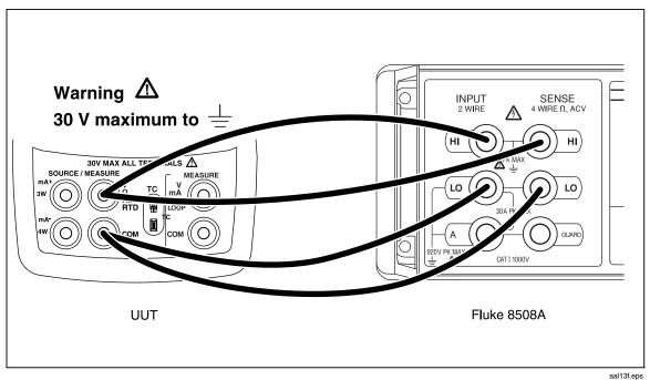
Figure 20. Ohms Hi Source Calibration Connections
