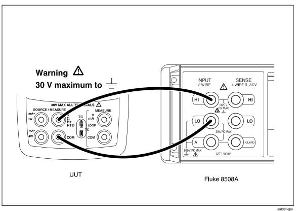
Figure 7. Lower Display Frequency Source Test Connections
