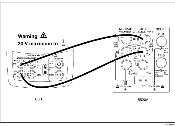
Figure 5. Lower Display mA Test Connections
