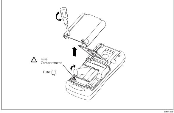
Figure 1. Replacing the Batteries and Replaceable Fuses
