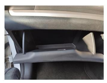
Typically, the evaporator and the in-cabin air blower are located behind the glove compartment, but it might be different depending on the make and model of your vehicle.
