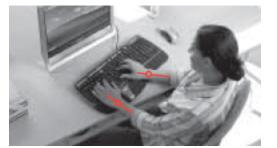
Figure 1. Overhead shot of split keyboard showing reduced ulnar deviation
