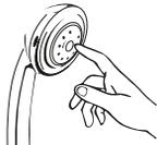
To remove mineral deposits simply glide your finger along the nozzle tips while the showerhead is running.
