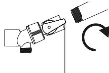
**2** Hand tighten Evolve Handshower Mount clockwise onto the shower pipe.
