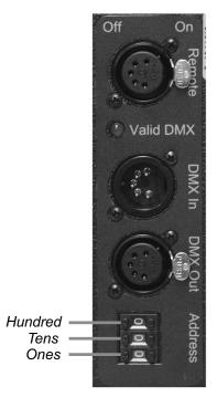
4) Plug the unit into a suitable power source. Turn the main power switch on and it will illuminate if power is present. The valid DMX light should also now be flashing. The unit requires about 7 minutes to heat before haze can be produced.
