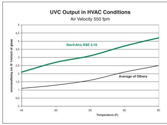
Steril-Aire's multi-patented UVC Emitter<sup>TM</sup> provides the best and longest-lasting UVC performance available. As shown in the comparison graph *(above)*, it has been independently tested to deliver an average of 5 times the output of other ultraviolet devices under HVAC operating conditions (45° F @ 550 fpm air velocity).
