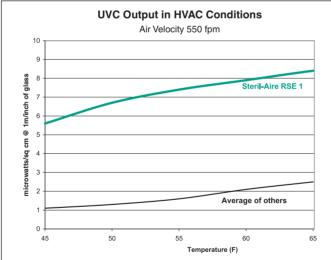
Steril-Aire's multi-patented UVC Emitter<sup>TM</sup> provides the best and longest-lasting UVC performance available. As shown in the comparison graph *(above)*, it has been independently tested to deliver an average of 5 times the output of other ultraviolet devices under HVAC operating conditions (45° F @ 550 fpm air velocity).
