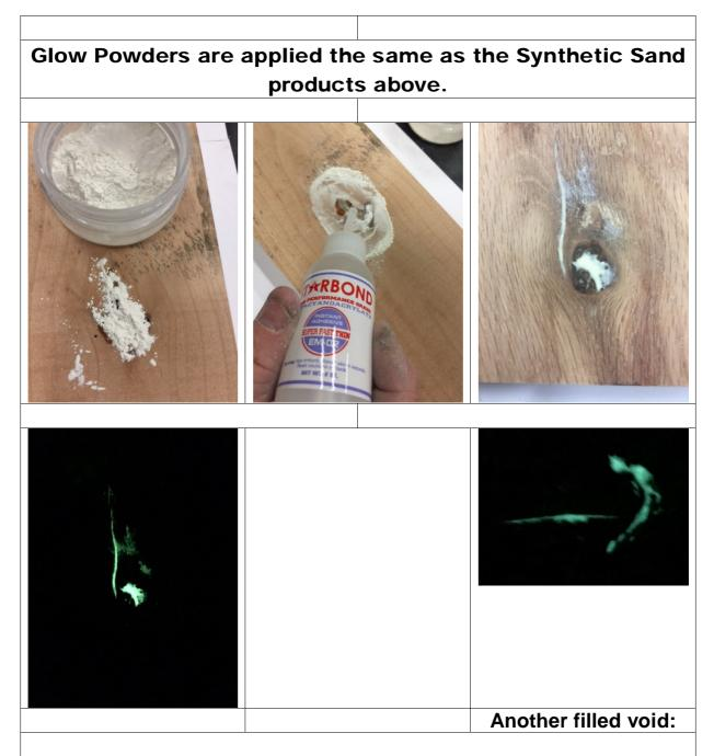
There are two main types of phosphorescent (glow) pigments: Jimmy Clewes Glow powders are a synthetic type of a phosphorescent pigment which is a grown crystal that is meticulously ground and treated. It glows 20-30 times longer than the other type on the market and has a much shorter excitation time (usually 20 minutes or less) for full glow. Sun Light or Fluorescent lighting is all that is required to activate this product.
