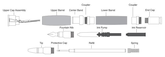
NOTE: Please do not press the front end of this kit with the tip removed. If you do so the parts will not assemble properly and you will void our warranty
