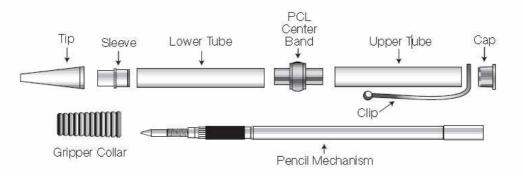
**Pencil Assembly** *Note: Line up parts according to layout above.*
