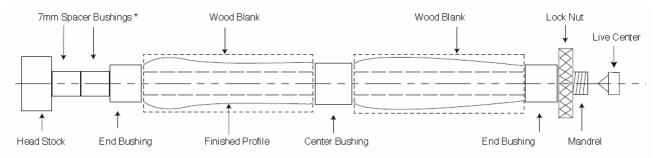
\* Note: The above diagram depicts a typical setup using mandrel and bushings. Turners using an adjustable mandrel will not need spacer bushings to secure the blanks.
