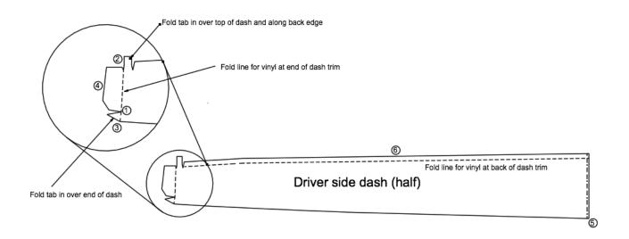
Installation of this vinyl kit should be performed with the front car doors open.
