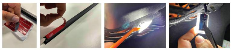
**Step 2.** Re-connect the OEM plug connector to the EVANNEX splitter plug connector. Then connect the OEM LED light to the black tip male plug on splitter connector. Push the OEM LED light with all cables back into its opening. Reach into the trunk liner to retrieve the white connector plug. Connect the white connector plug to the Trunk Interior White LED Strip connector. Bundle and fasten the extra white cable. Then hide cable behind the trunk liner.
