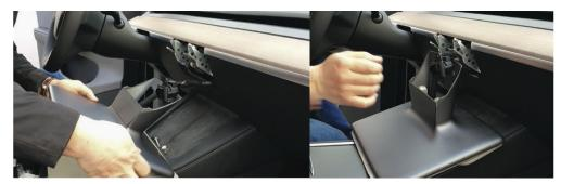
5. Make sure you place the screen on top of the provided foam pad or any soft fabric to protect screen surface.
