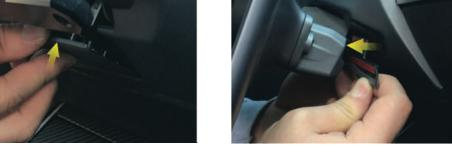
9. Fasten the temperature sensor cable to the new temperature sensor base plate with the provided small screws. Push in plate until it snaps in place. Make sure to install the correct base plate for your Tesla model.
