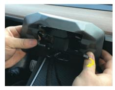
3. Slide mount protective cover on one side of the mount and then rotate the swivel mount to be able slide the other side in. Be sure to feed all cable through the mount protective cover hole.
