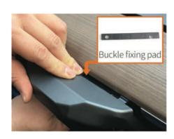
4. The buckle gasket/pad is used if the gap between the protective cover and the dash is significant. If the gap is normal there is no need to use the buckle gasket/pad.
