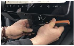
2. Remove the temperature sensor with 3. Remove the original car screen the provided torx key or on other models bolts with a 10mm socket wrench. pull on both tabs to release sensor.
