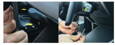
8. Carefully install the screen with the provided H5 hexagon socket bolts. Do not let go of the screen until bolts are fasten.
