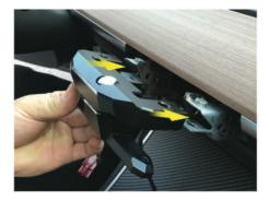
1. Insert the black rotating mount in to the OEM screen bracket.
