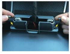
7. Fasten the plastic protective cover with the OEM screws using the provided torx tool.
