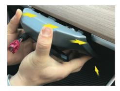
5. Push in the plastic cover until it snaps in place, make sure bottom tabs snap in place as well.
