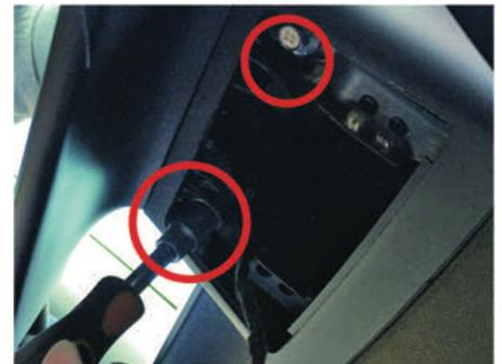
3. Remove the original car screen bolts with a 10mm socket wrench. (Save bolts for later)
