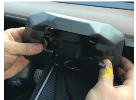
3. Slide mount protective cover on one side of the mount and then rotate the swivel mount to be able slide the other side in. Be sure to feed all cable through the mount protective cover hole.
