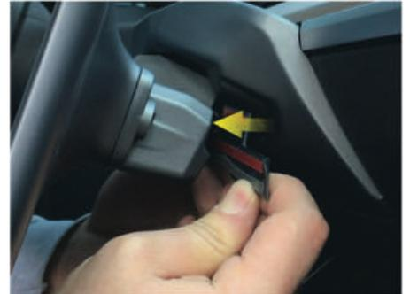
10. Remove the double sided tape on the back of the protection sheet and press into place. Your installation is now complete..
