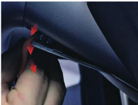
1. Remove the temperature sensor cover plate with the provided wedge tool.
