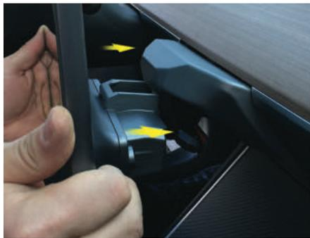
8. Carefully install the screen with the provided H5 hexagon socket bolts. Do not let go of the screen until bolts are fasten.
