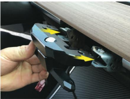
1. Insert the black rotating mount in to the OEM screen bracket.
