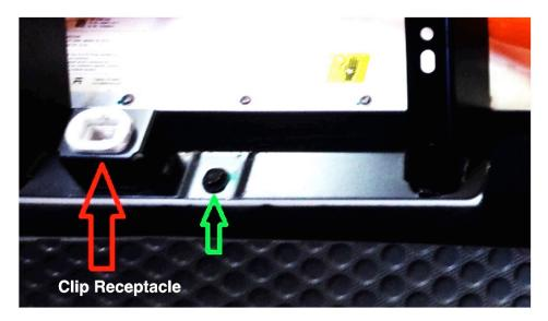
The clips are difficult to remove; however, they can be detached by exerting <u>heavy upward force</u> at the site of the fastener and on the side of the seat cushion, one clip at a time. DO NOT twist the seat as you pull upward. The same operation is applied for the second fastener.
