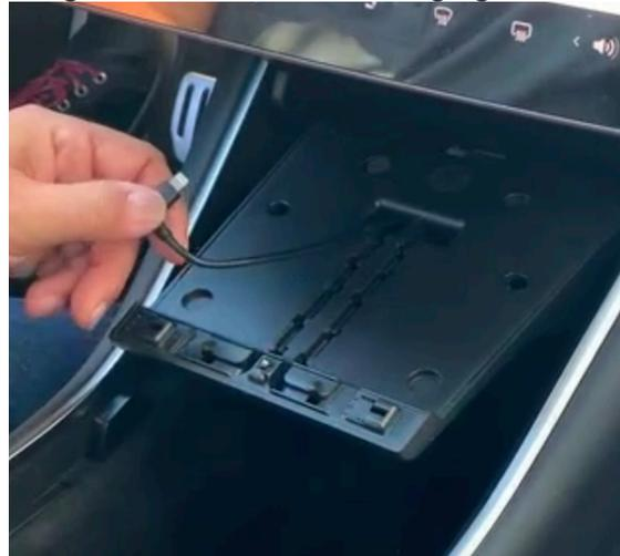
**Step 4. Remove EVANNEX Dual Qi Wireless Charging Pad from its box. Thread the cables through the opening in the OEM charging shelf.**
