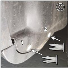
**FIGURES D** Place mud flap logo-side facing rear of vehicle against lower mounting points. Install SCREW .5BLKSS and WASHER SMWASH through mounting points 1, 2. Do not fully tighten.
