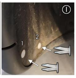
**FIGURE J** Place mud flap logo-side facing rear of vehicle against corresponding lower mounting points. Install SCREW & WASHER through mounting points 1, 2. Do not fully tighten.
