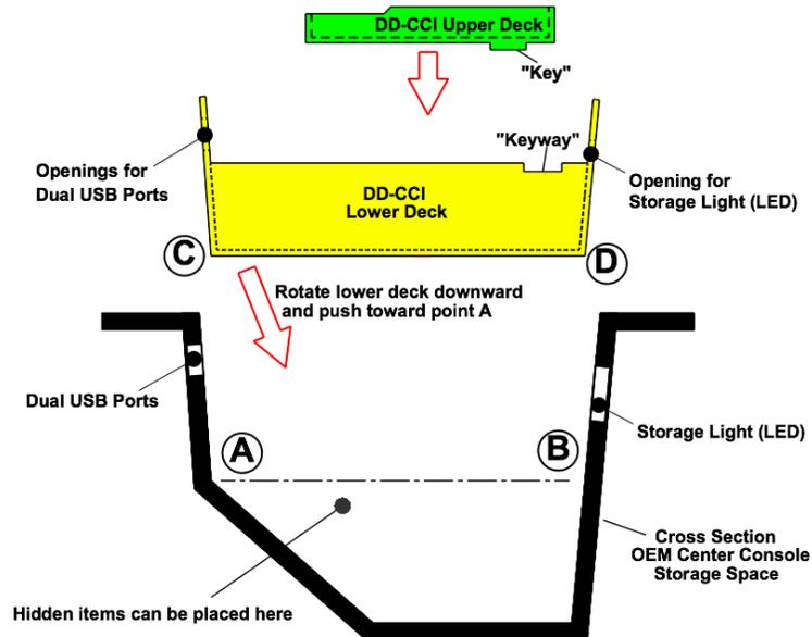
Figure 1. Installing the DD-CCI
