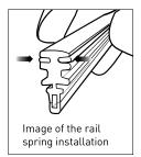
② Attach the end clip to the rail spring in the right direction.
