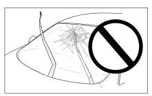
1) Make sure that the wiper arms do not make contact with the windshield while the wiper is being replaced. It can break the windshield.
