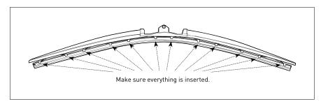
④ Push the end clip until it is inserted all the way.
