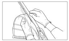
2) When the wiper or water repellent coating does not seem to work well, clean the windshield and wiper blade and operate the wiper for 3-5 minutes on a completely dry surface before use.
