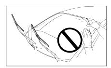
4) Do not attach any kind of glass coating, chemical substances, or films on to the surface of the windshield. It can cause wiper noise or shaking.
