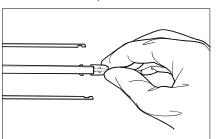
② Remove both the rail spring and the end clip.
