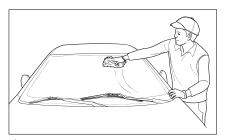
1) Before installing the wiper for the first time, clean the car windshield and operate the wiper for 3-5 minutes on a dry surface before use.
