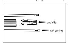
[Order] 1. First, remove the rail spring. 2. Remove the end clip.
