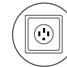
NEMA 14-50P 240V outlet Ground facing down Or electrical material to hardwire
