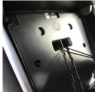
**Step 2. Rotate the OEM charging shelf downward and remove the OEM light grey, rubberized charging platform cover by pulling it upward.** We recommend storing it in a safe place.
