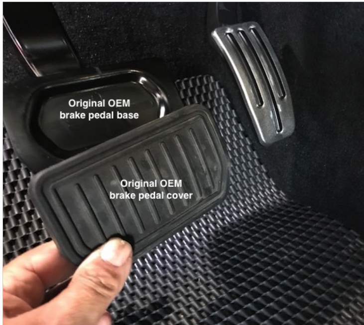
Photo # 3 Remove OEM Brake Pedal cover to expose base
