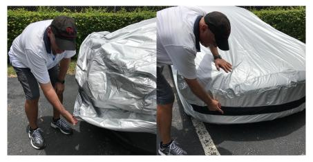
Step 5. Pull the rear of the Car Cover over the rear end of the Model 3 using the elastic bottom to anchor it under the rear bumper area.
