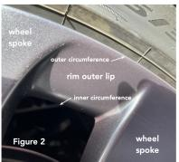
rim. The accent edge should align with the beginning of the radius of the outer circumference of the rim edge (Figure 3, shows 21-inch wheel). Smooth the remainder of the accent
