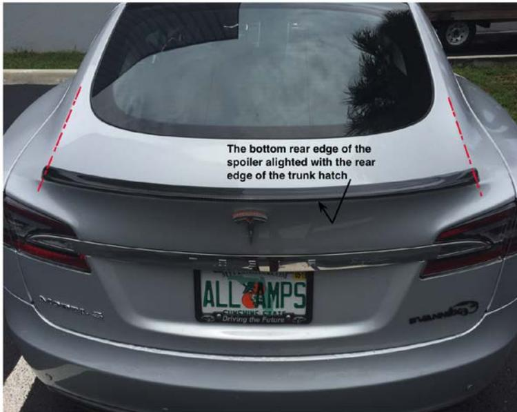
Figure 1. Overall alignment of Spoiler on trunk hatch
