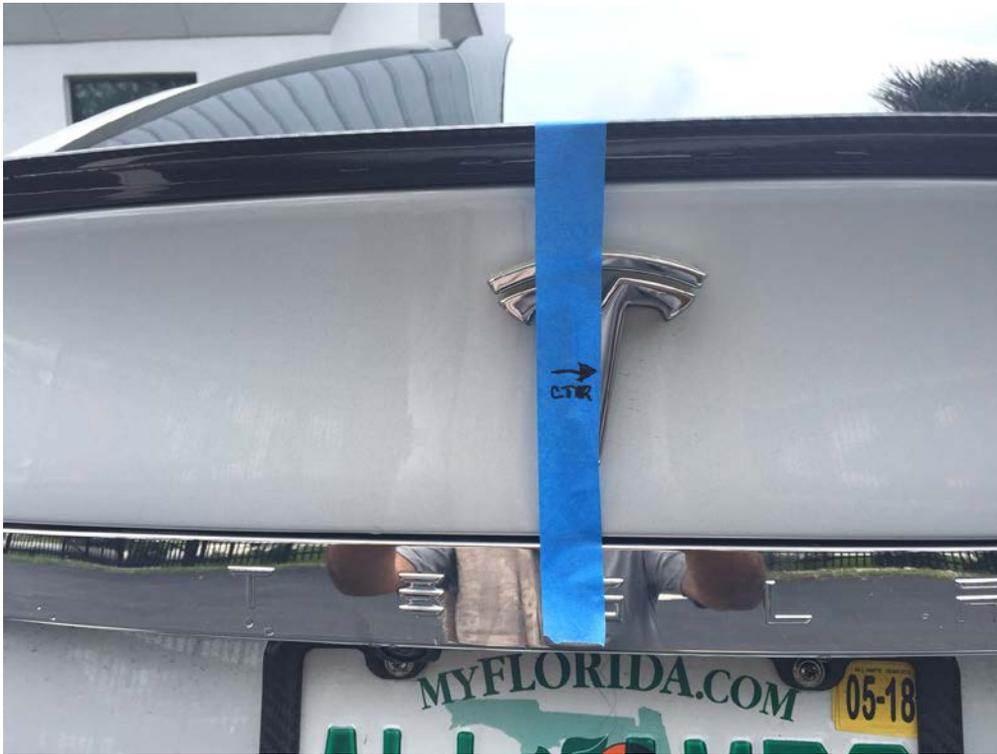
Figure 4. Use tape to identify spoiler centerline
