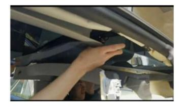
6) Open the interior trim panels on both sides and fold down the rear seats. Note: the film side of the electronic skylight card plate should be facing up, the card plate is moderately bent and placed in the card slot between the glass and the car body, and pushed to the front of the car in place.
