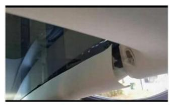
7) First, install the caulking strips for the finished product into the steel channel of the original car at the rear left side of the car and then clip the sky curtain into the place where the caulking strip is located, that is into the steel channel of the original car. Tesla does not have glass glue, so the canopy will collapse after installation, and the caulking strips are used to clamp the canopy left and right so that the canopy will not collapse.
