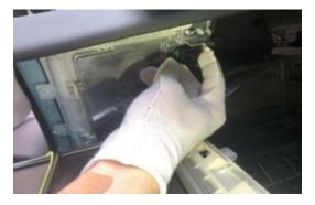
3) The silver trim strip can be removed directly after removing the screws with T20 torx screwdriver.
