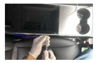
4) Remove the cup holder cover. If there are no screws on the four corners of the cup holder, just lift the whole cover. If the four corners of the cup holder are fixed with screws after removing the cover, just lift the cup holder directly after removing the screws.
