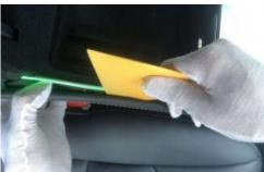
2) Lift up the front wireless charging part and remove the wireless charging plug.
