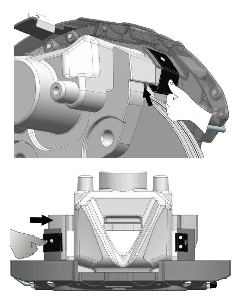
Note: Make sure bracket is even on both sides and align caliper cover center with the caliper center.
