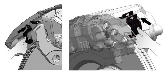
**Step 6.** Thread the hexagon bolt through the buckle hole. Then, attach the provided nut to fasten buckle.
