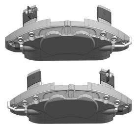
Note: The front wheel caliper covers are larger than the rear wheel caliper covers.
