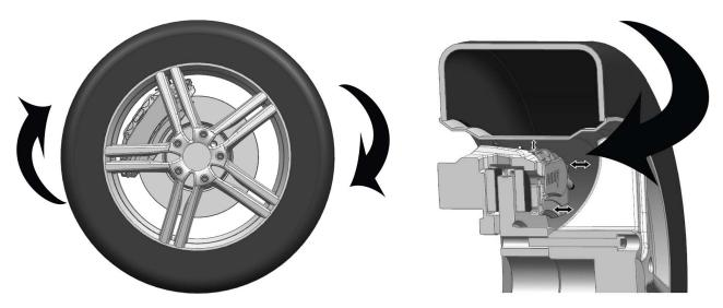
After confirming that there is no problem. Install remaining lug nuts. Jack down vehicle and complete securing lug nuts with the appropriate tool.
