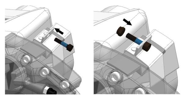
**Step 7.** Tighten the bolt and the nut with the provided tools. Make sure to apply enough force to secure them in place.
