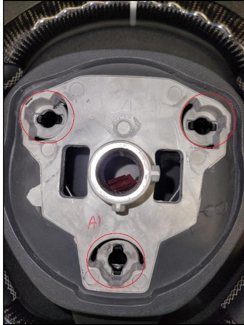
(Referenced image showing back of steering wheel core and location of tabs to be removed from locked position)
