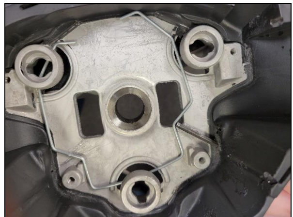
(Internal view of the formed wire being released inside of steering wheel)
