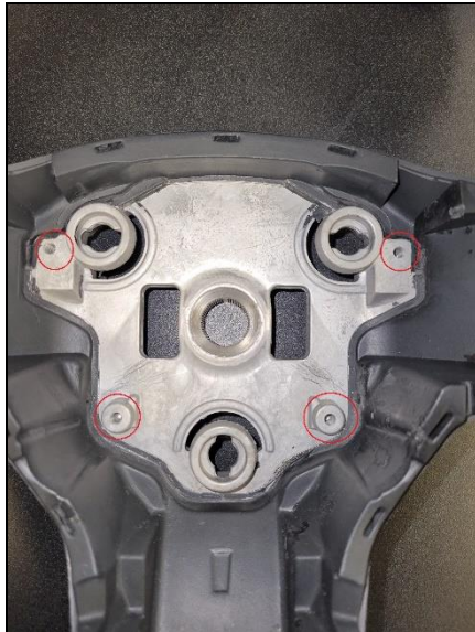
(Reference of where T25 Torx Screws are located with/without hardware within steering wheel core)
