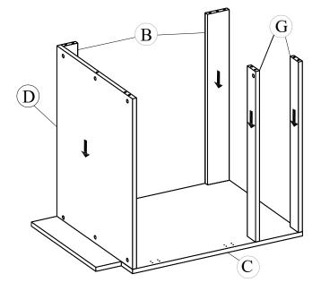
Step~4 Insert the next Left Side Panel Locking the cam locks by turning them 180° clockwise. \* Left side panel (A)
