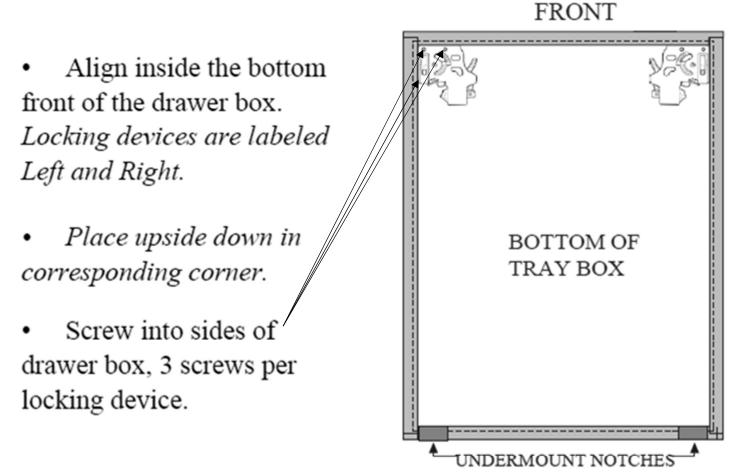
*Tip:* Avoid screwing the devices into the bottom of the tray box to keep the screws from puncturing the tray box
